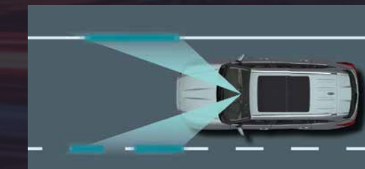
LANE KEEPING SYSTEM
